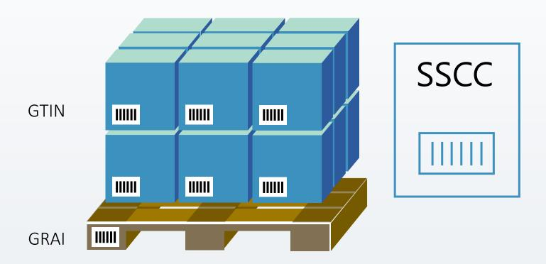
Serial Shipping Container Code can be used by companies to identify a logistic unit, which can be any set of trade items packed together for storage and/or transportation purposes; for example, a case, pallet or parcel.
